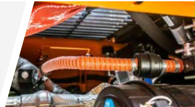
Heavy-duty filtration system (ejector)
