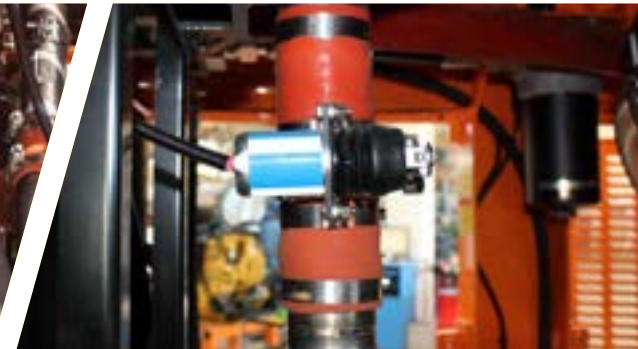
Air shutoff valve
